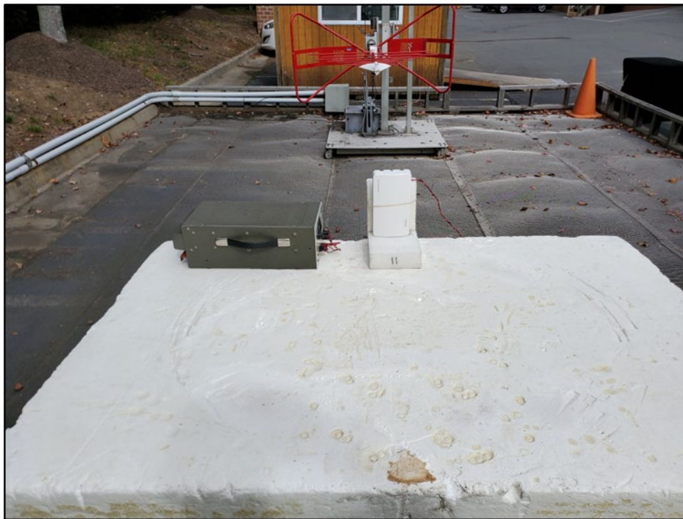
Photograph 1: Radiated Emissions Testing – Front View (Unintentional Emissions, <1 GHz)
