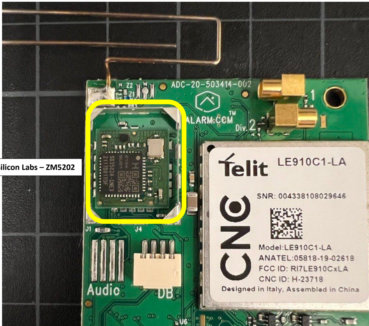
ADC-SEM-300 – Photo 10 – Top PCB – Top View No Shields; Z-Wave Module Zoomed
