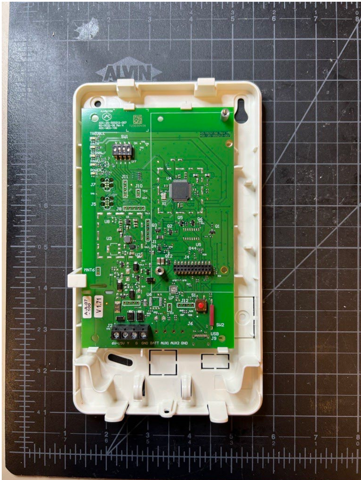
ADC-SEM-300 – Photo13 – Top View of Bottom PCB in Chassis after Top PCB Removed
