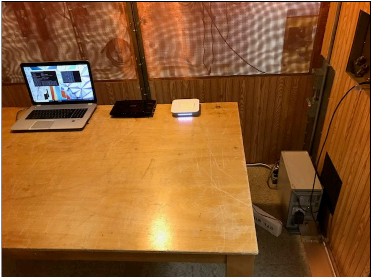
Photograph 5: Conducted AC Emissions Testing – Front View
