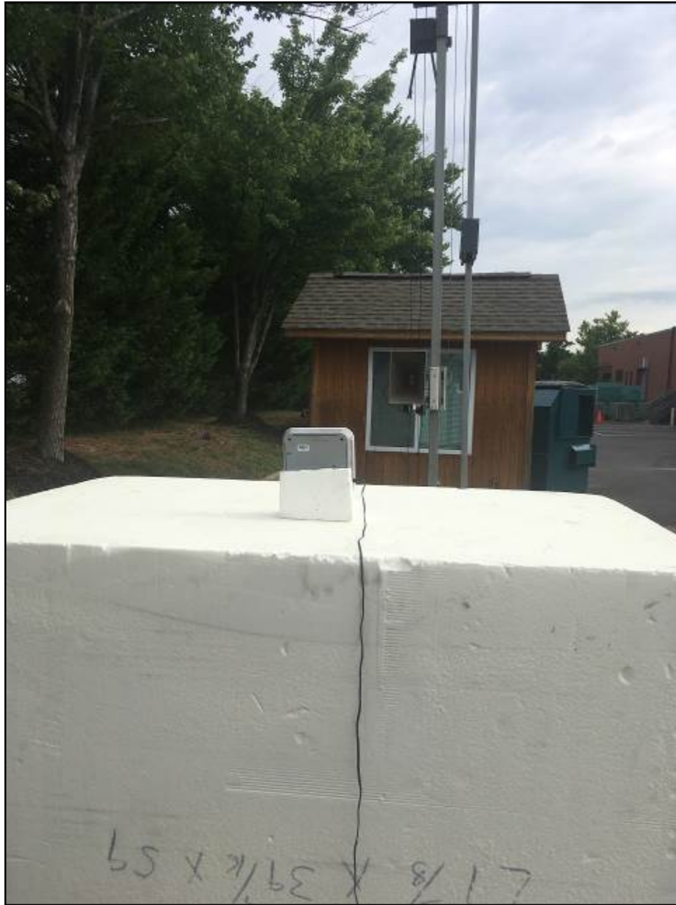
Photograph 4: Radiated Emissions Testing – Back View (Spurious Emissions, >1 GHz)
