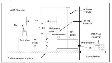
Radiated measurements setup f > 1-18 GHz
