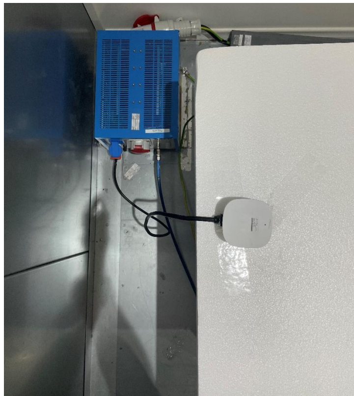
Figure B6. Conducted Emission test setup
