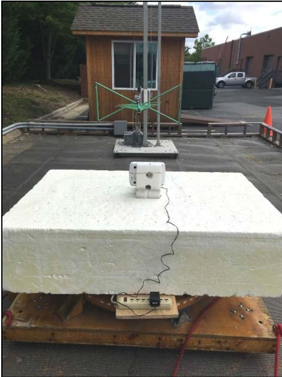
Photograph 2: Radiated Emissions Testing – Back View (Digital Emissions, <1 GHz)
