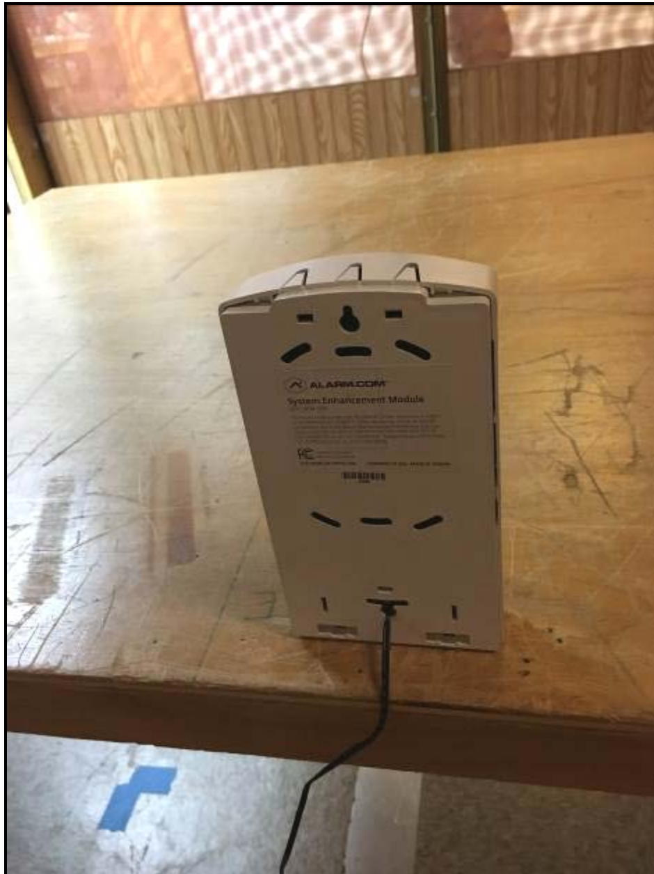
Photograph 6: Conducted Emissions Testing – Back View
