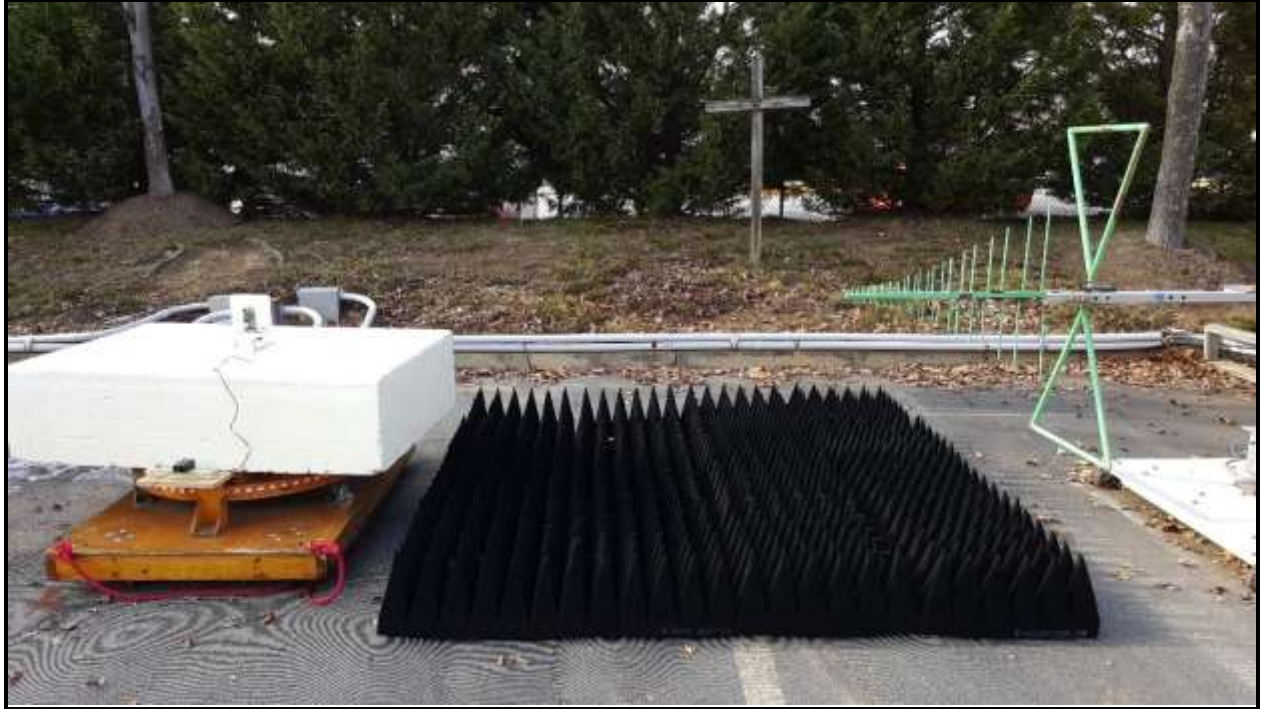
Photograph 4: Radiated Emissions Testing
