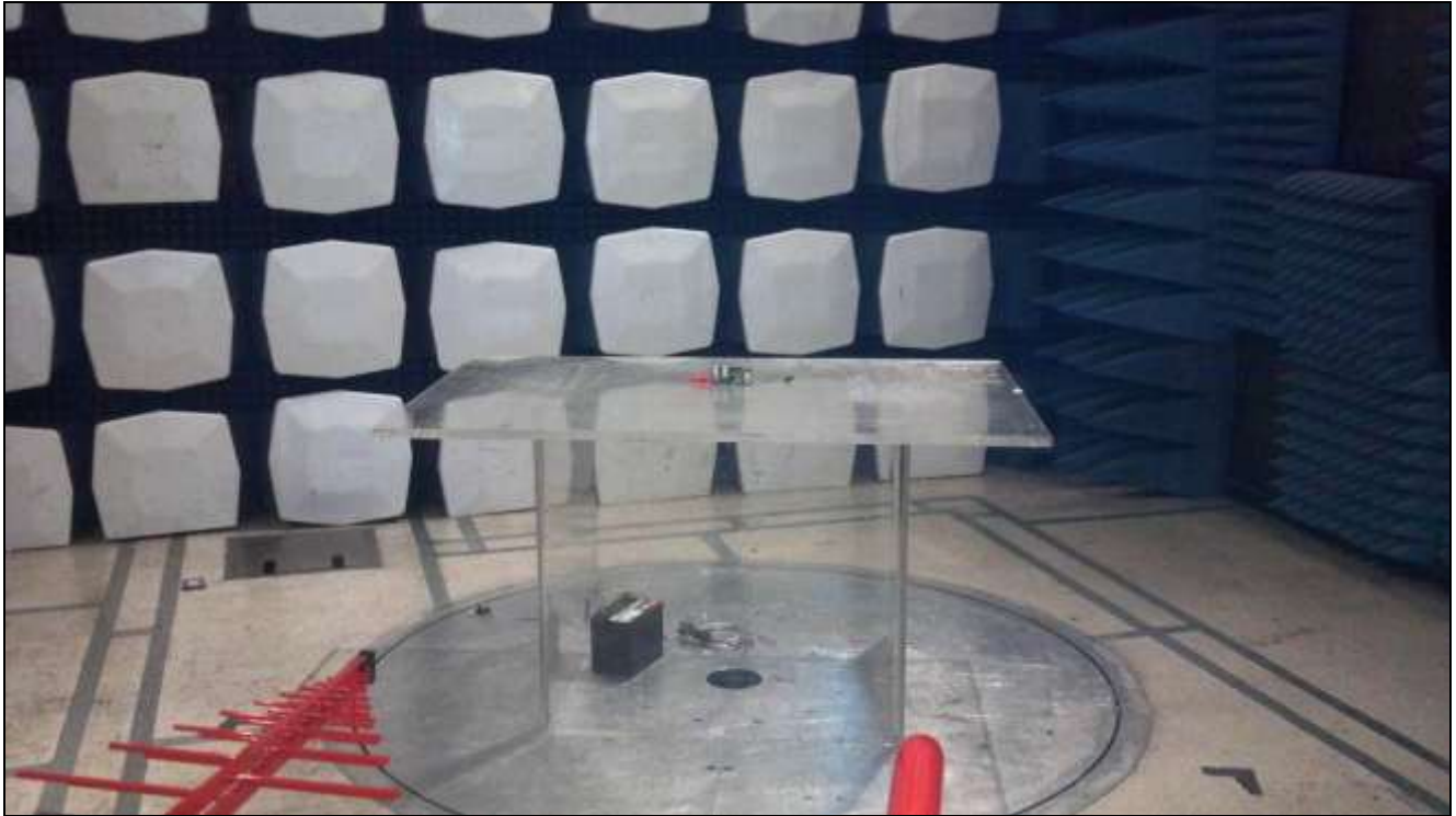
Photograph 2. Radiated Emission, Test Setup
