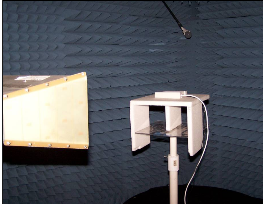
Photograph 6. Transceiver Spurious Emissions, Test Setup
