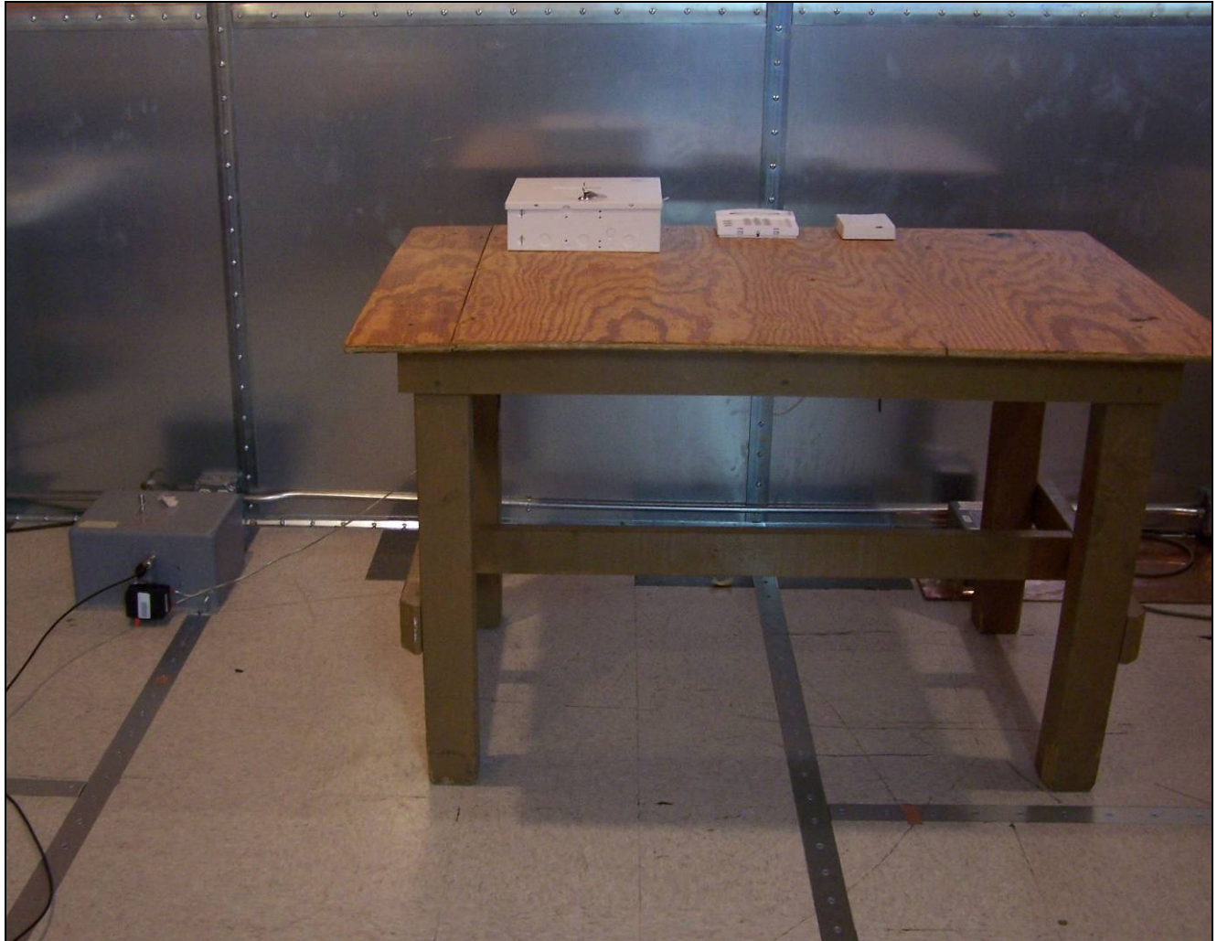
Photograph 5. Conducted Emissions, 15.207, Test Setup
