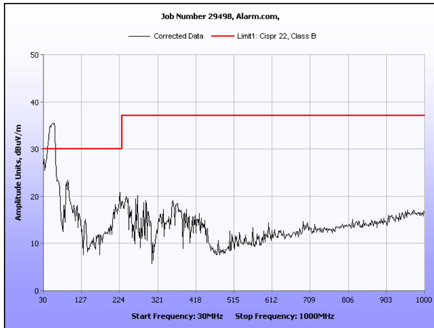
Plot 4. Radiated Emissions, Pre-Scan, 30 MHz – 1 GHz, ICES-003 Limits
