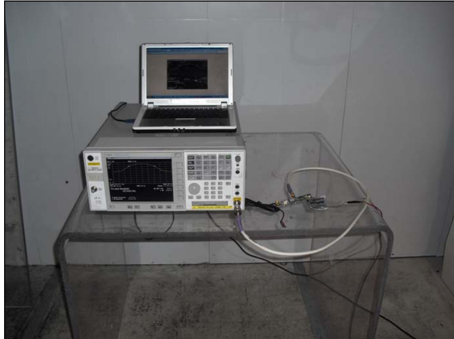
Photograph 5. Occupied Bandwidth, Test Setup
