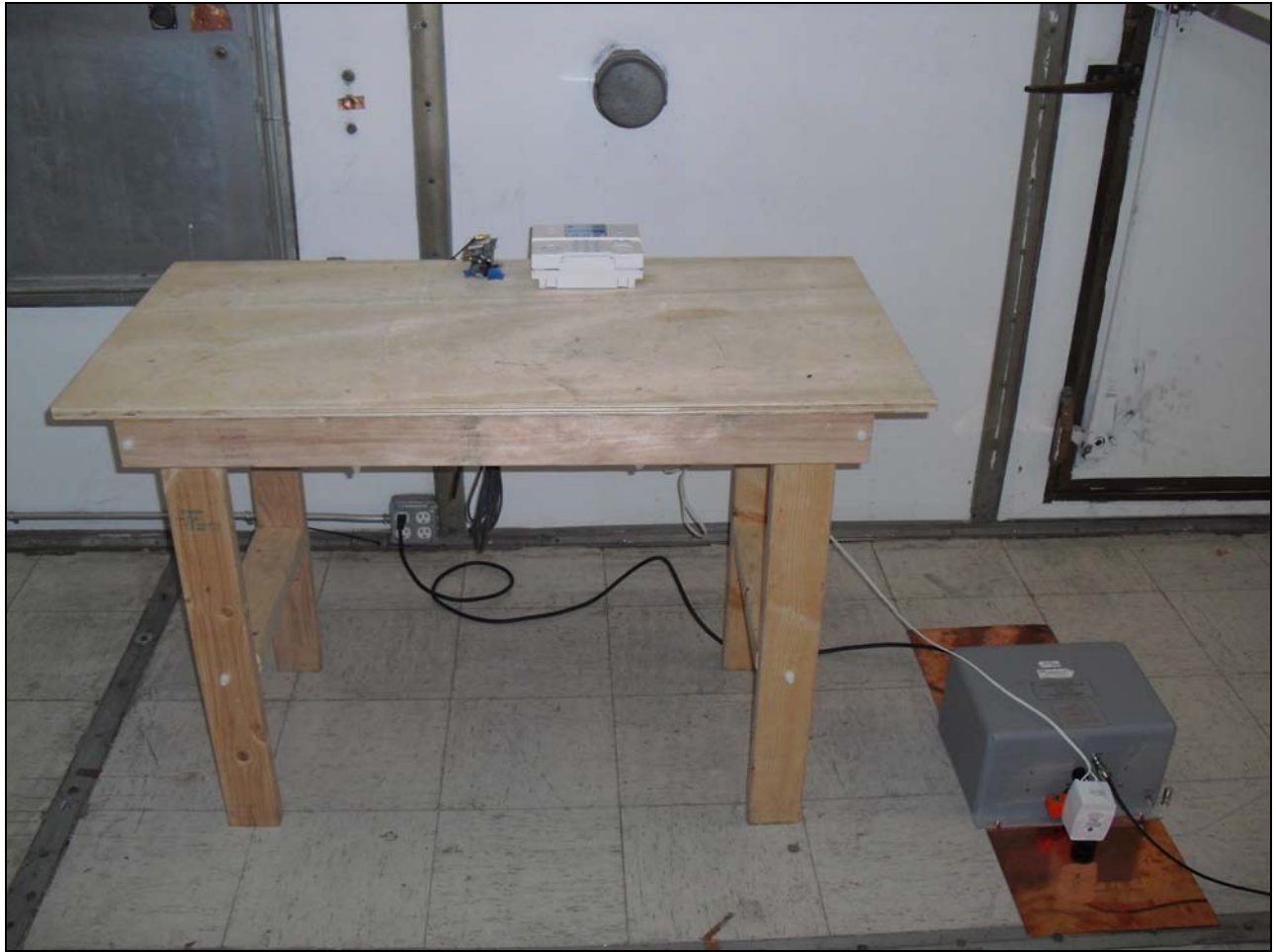
Photograph 4. Conducted Emissions, 15.207, Test Setup
