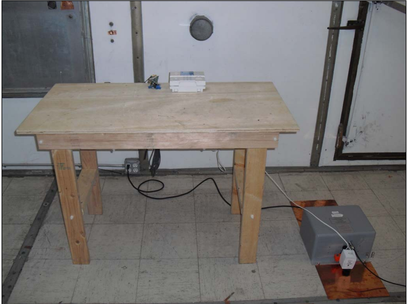
Photograph 2. Conducted Emissions, Test Setup
