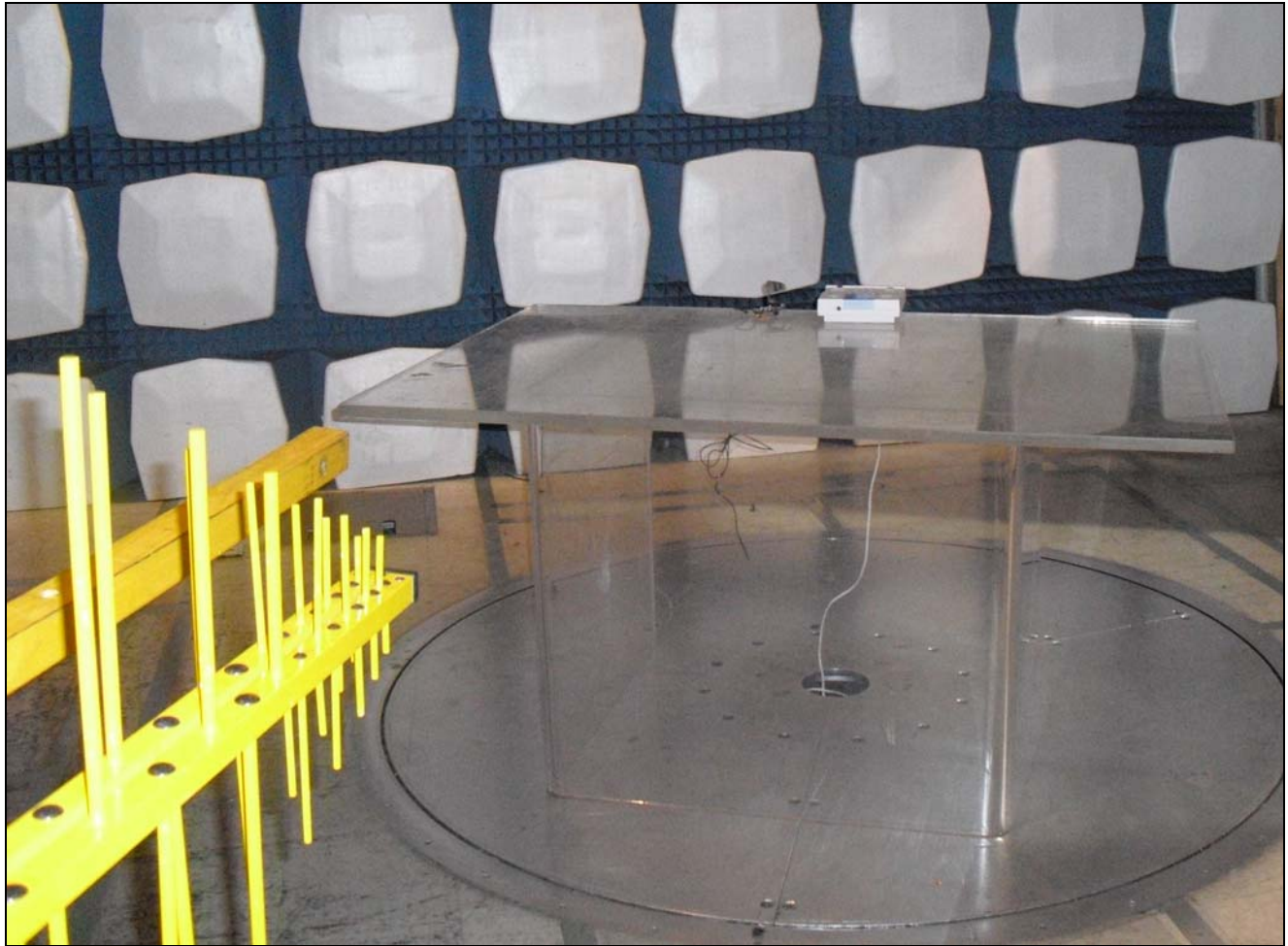
Photograph 3. Radiated Emissions, Test Setup
