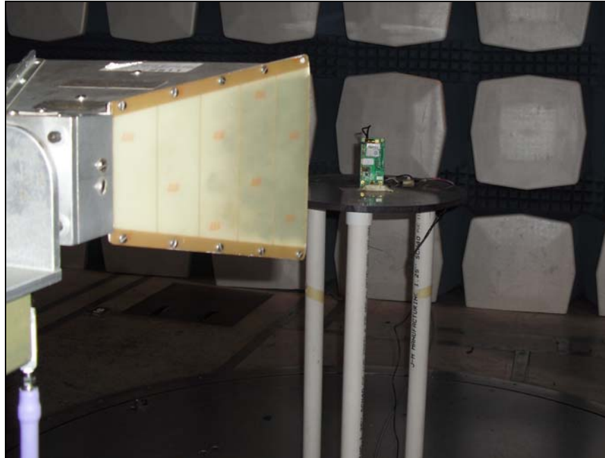
Photograph 6. Transceiver Spurious Emissions, Test Setup
