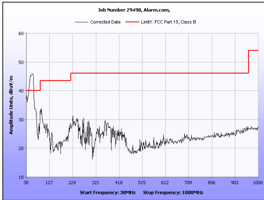
Plot 3. Radiated Emissions, Pre-Scan, 30 MHz – 1 GHz, FCC Limits
