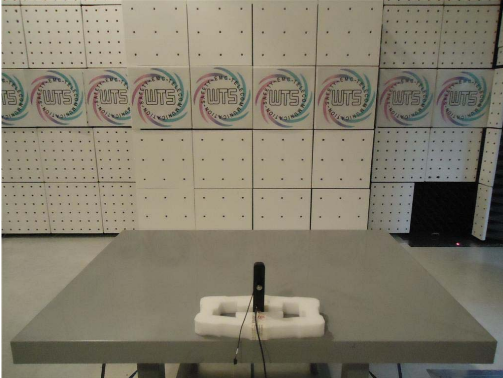
Set Up Photo of Conducted Emission
