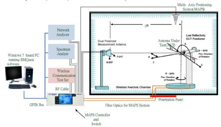
Theta is the spherical axis that rotates along the Cartesian Y axis while Phi is the spherical axis that rotates along the Cartesian Z axis. The initial measurement position (Theta =  $0^{\circ}$  and Phi =  $0^{\circ}$ ) is illustrated in each of the test setup photographs. The EUT has only one mechanical configuration each and it was tested in the Free-space configuration, whereby the EUT has been placed directly on a support.
