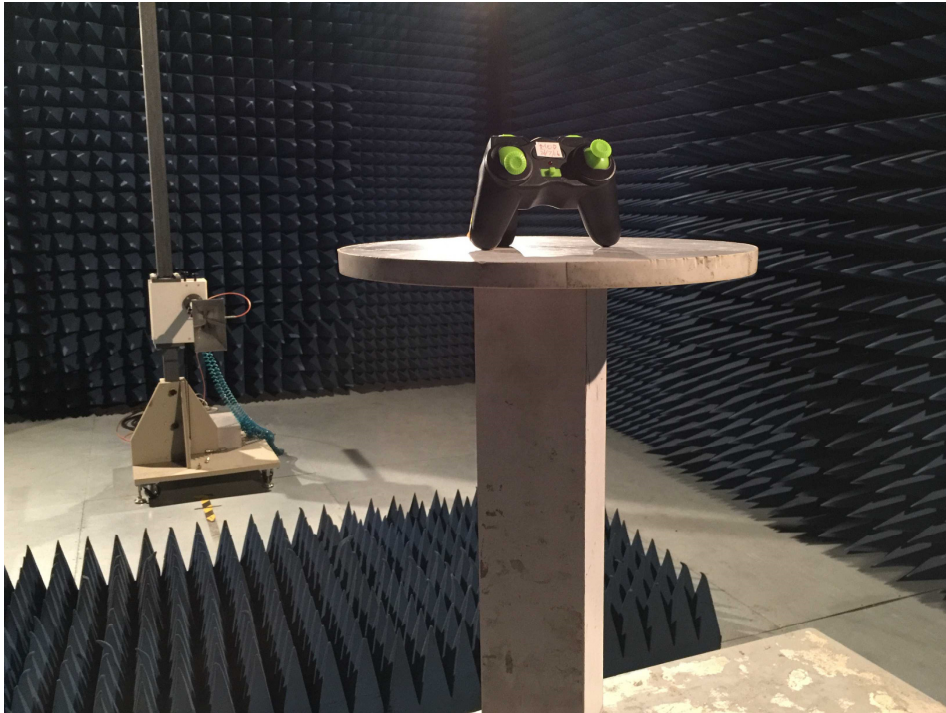
Setup for radiated emission
