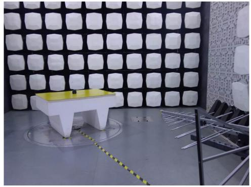
8.2 Radiated Emissions(30MHz-1GHz) Test Setup
