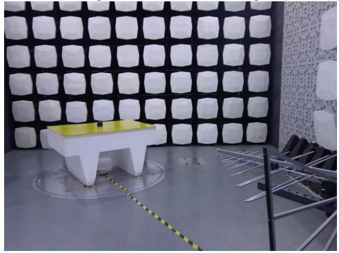
1.2 Radiated Emissions(30MHz-1GHz) Test Setup
