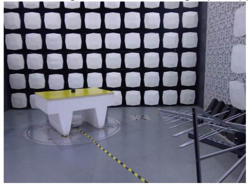
1.2 Radiated Emissions(30MHz-1GHz) Test Setup
