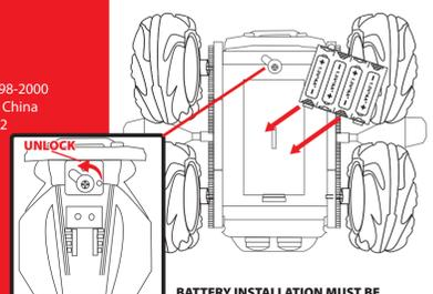
**BATTERY INSTALLATION MUST BE PERFORMED TWICE, ONCE ON EACH SIDE**
