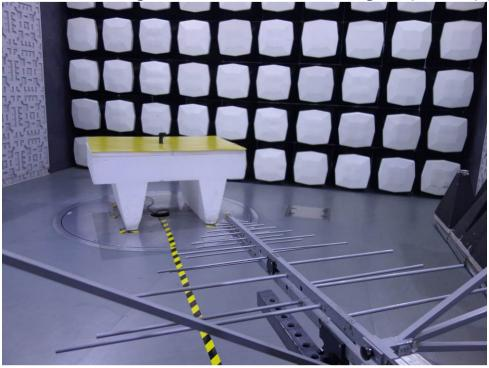
1.2 Radiated Emissions(30MHz-1GHz) Test Setup
