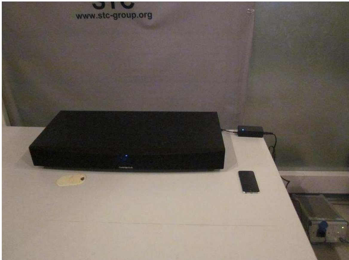
Measurement of Conducted Emission Test Set Up
