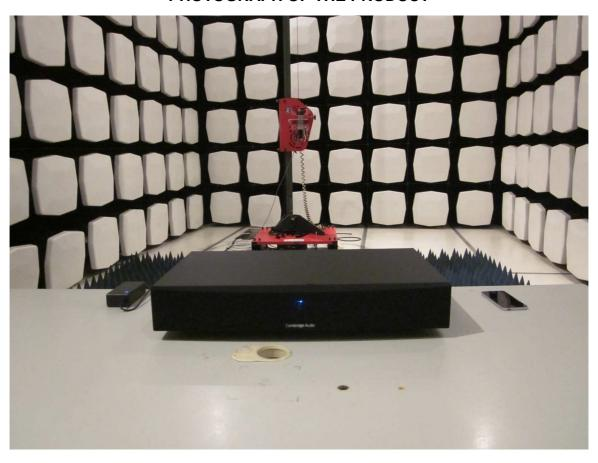
**Measurement of Conducted Emission Test Set Up**
