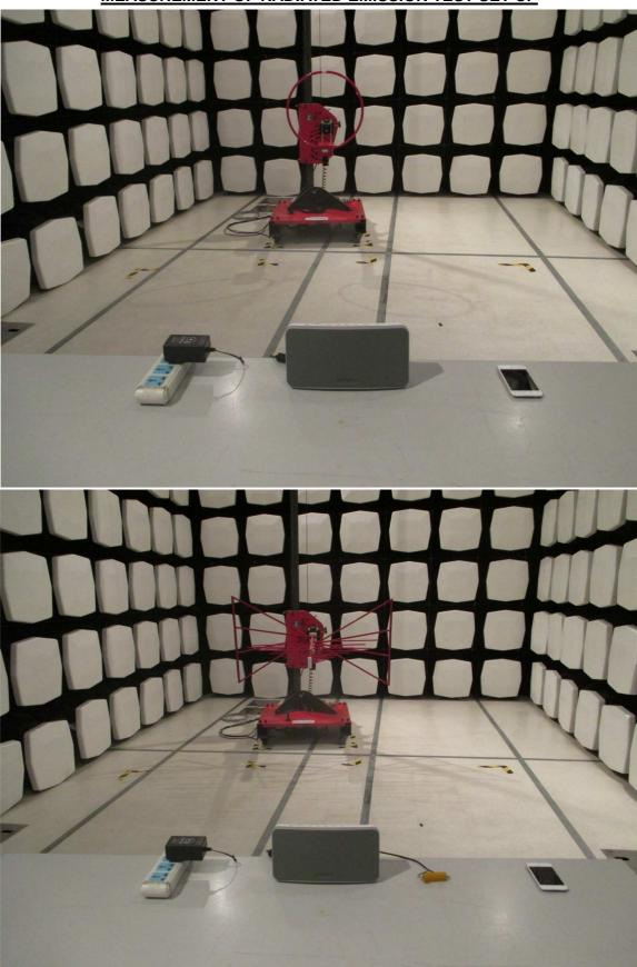
MEASUREMENT OF RADIATED EMISSION TEST SET UP
