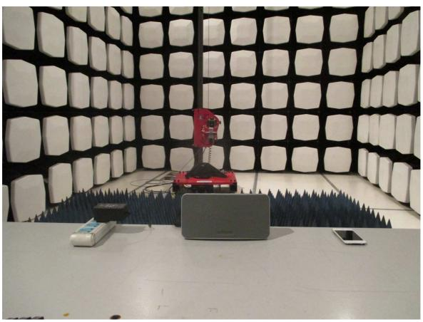
MEASUREMENT OF CONDUCTED EMISSION TEST SET UP
