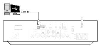
The Edge NQ USB Audio input is intended to connect directly to a PC or Mac computer. The Edge NQ configuration is USB Audio profile
