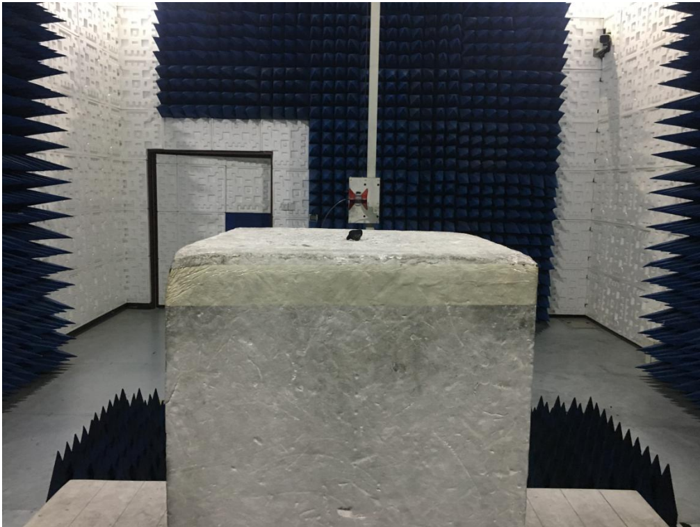
RADIATED EMISSION TEST SETUP ABOVE 1GHZ
