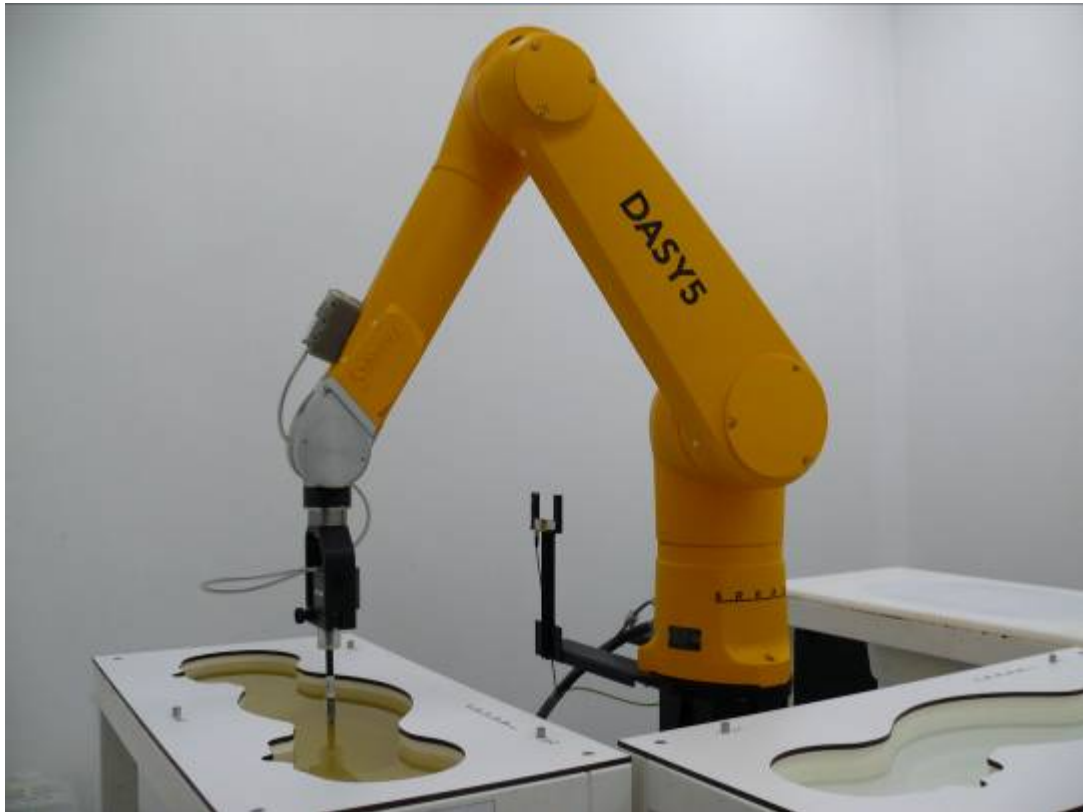
Picture 2: Specific Absorption Rate Test Layout
