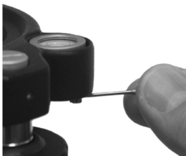
Fig. 4-51 Circular Level adjustment
