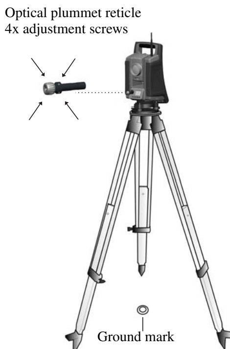
Fig. 4-50 Optical plummet adjustment
