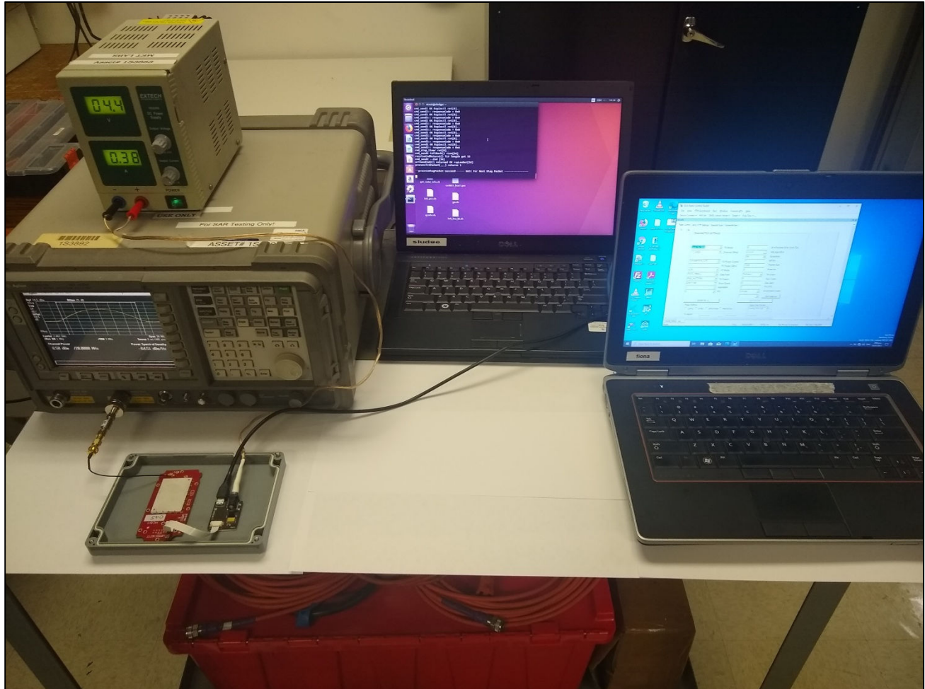
Conducted Measurement Test Setup
