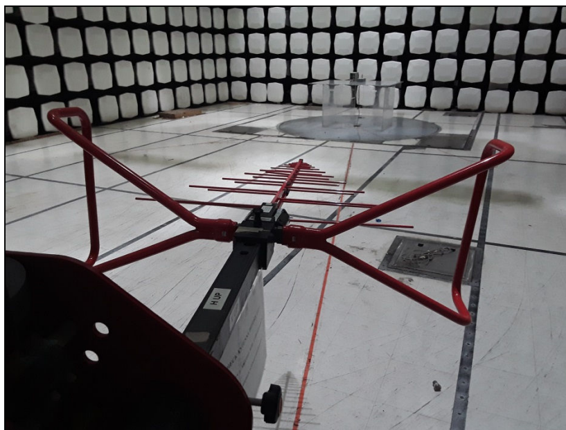
Photograph 1. Radiated Spurious Emissions, Below 1 GHz, Test Setup
