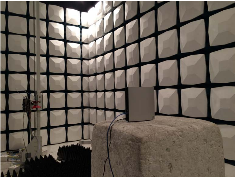
Description: Radiated Emission Test Setup for 1~18GHz
