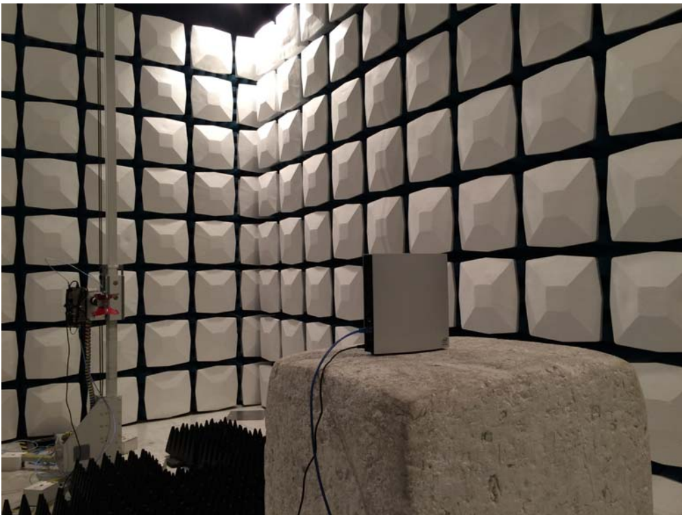
Description: Radiated Emission Test Setup for 1~18GHz
