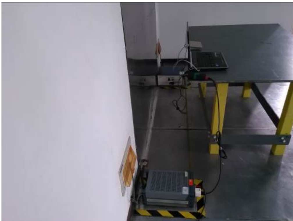
Conducted Emissions Test Setup Side View-Adapter: RD1200500-C55-8MG
