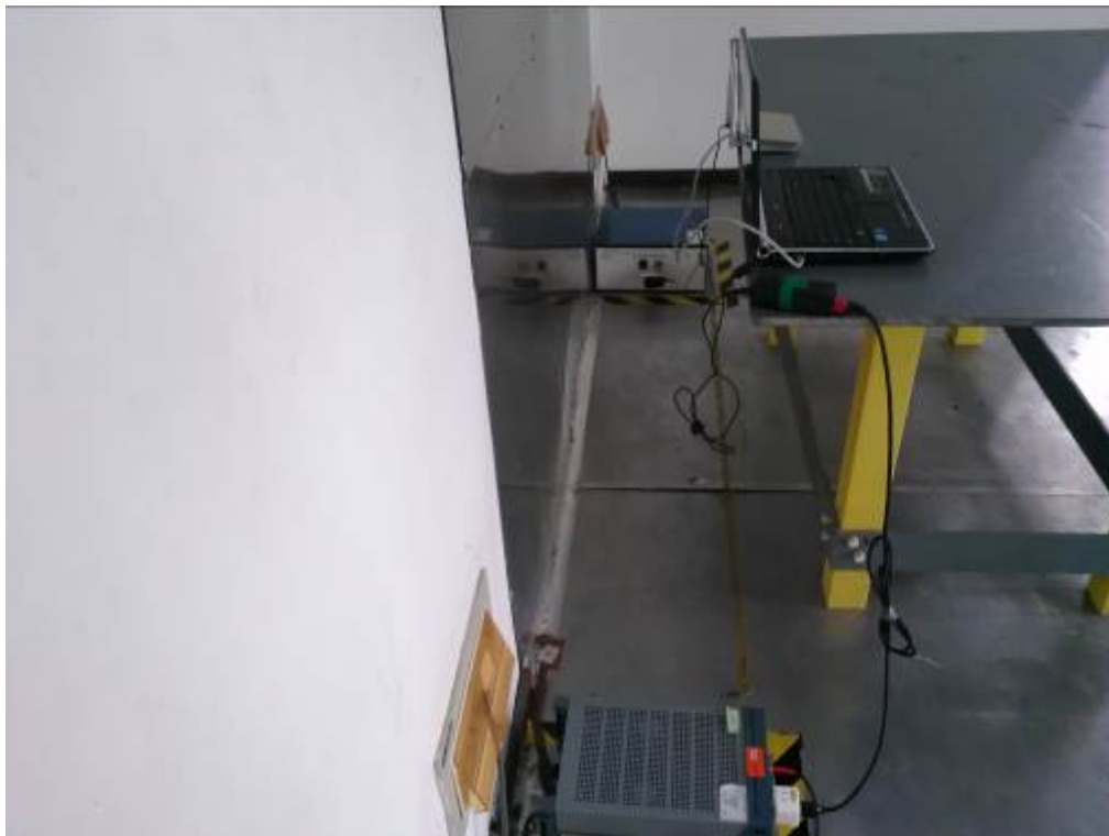
Conducted Emissions Test Setup Side View-Adapter: PSAA06A-120
