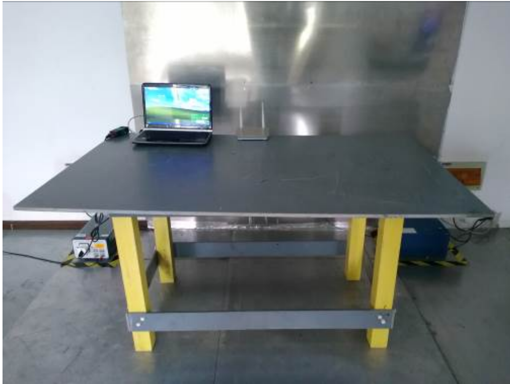
Conducted Emissions Test Setup Front View-Adapter: PSAA06A-120
