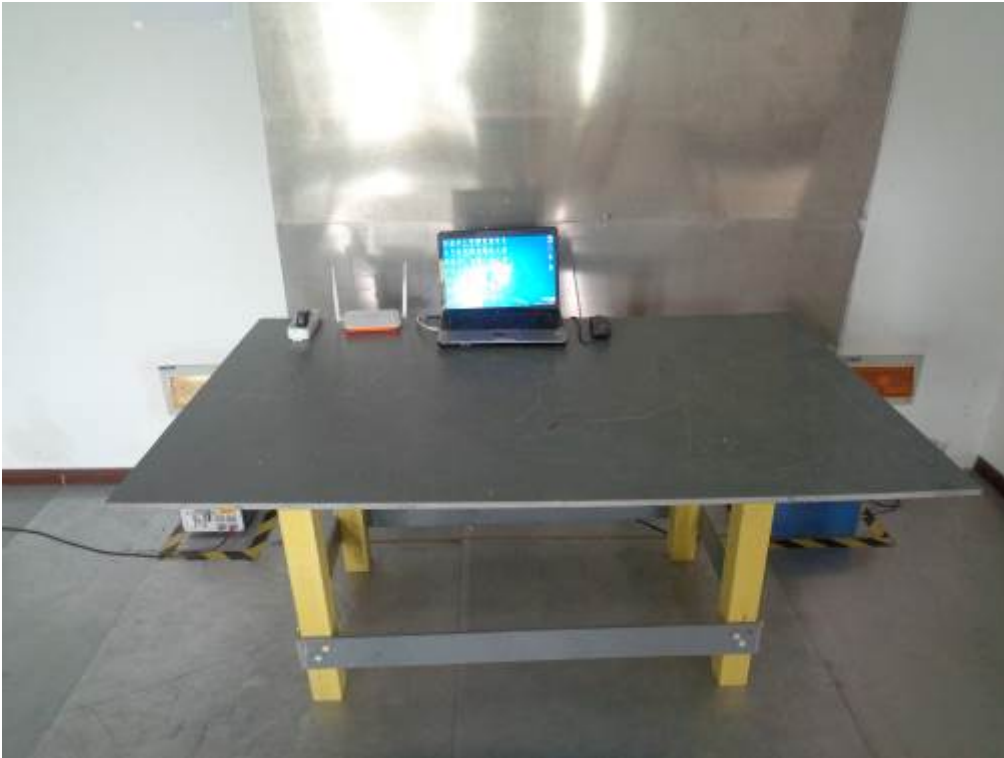
Conducted Emissions Test Setup – Front View
