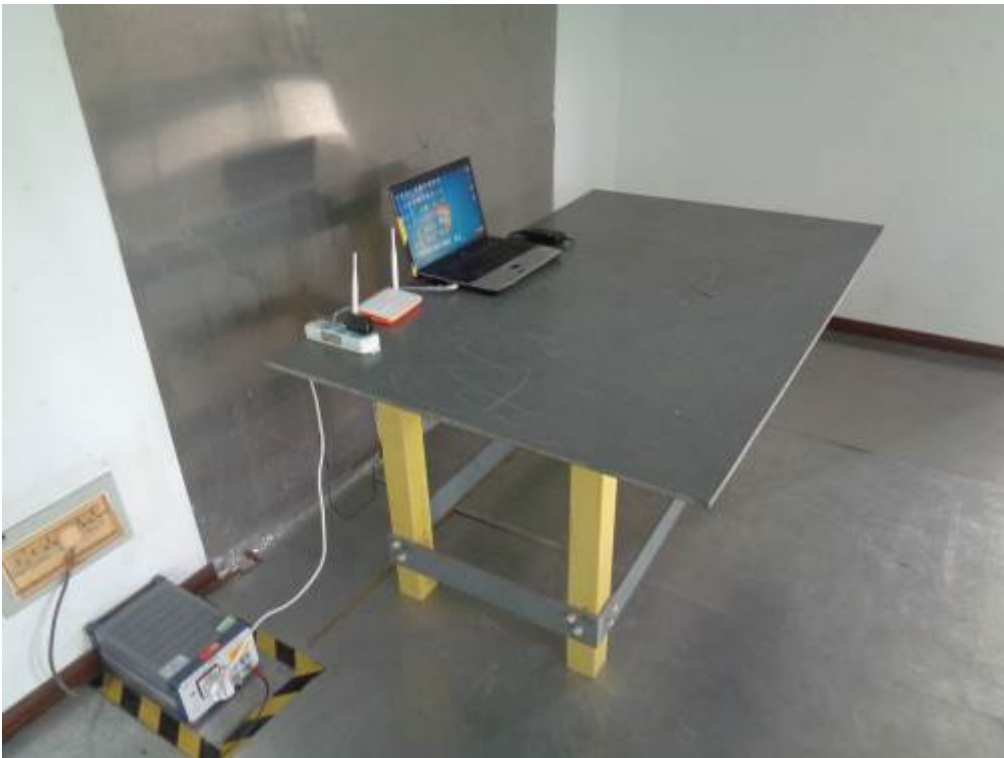
Conducted Emissions Test Setup – Side View
