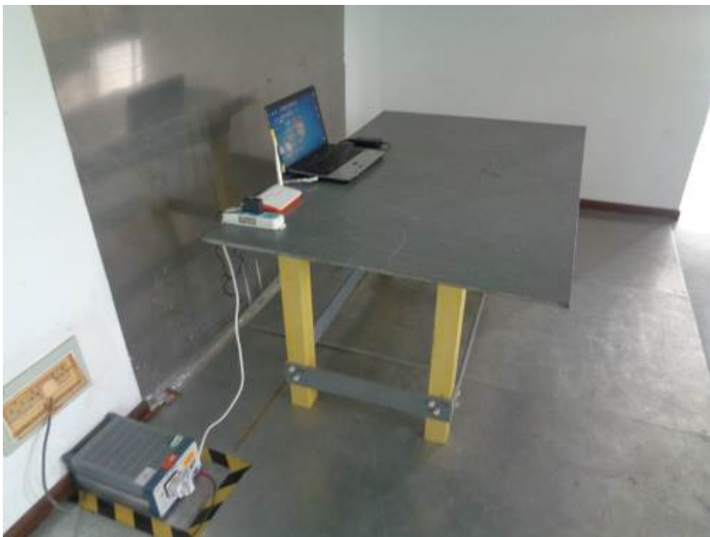
Conducted Emissions Test Setup Side View
