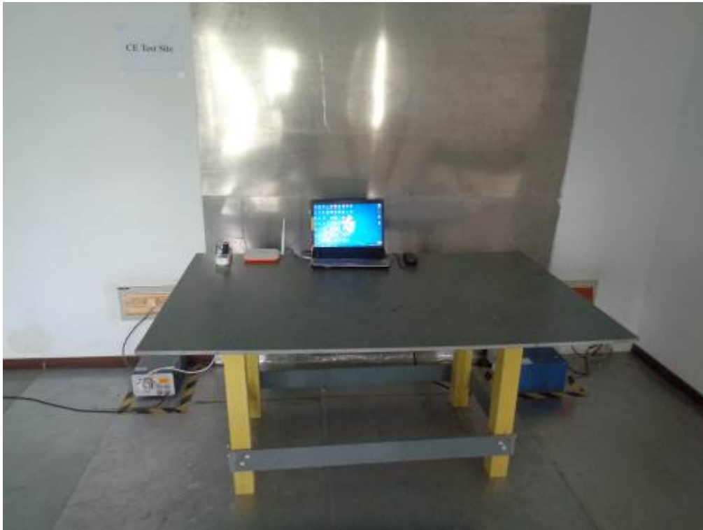
Conducted Emissions Test Setup Front View
