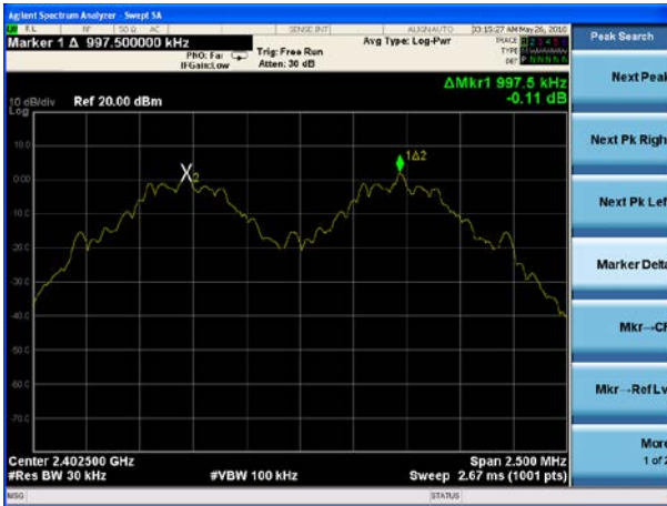
(1Mbps) Channel Separation plot on channel 39-40
