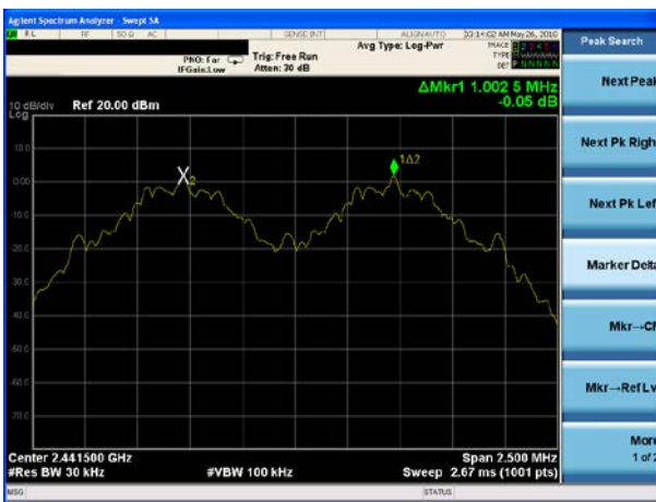
(1Mbps) Channel Separation plot on channel 39-40
