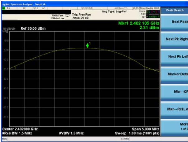
Peak output Power plot on channel 39 (1Mbps)
