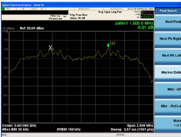
(3Mbps) Channel Separation plot on channel 77-78
