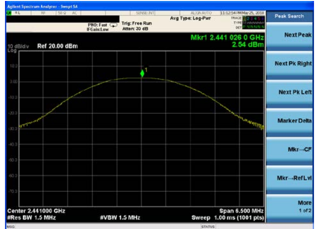
Peak output Power plot on channel 78 (2Mbps)
