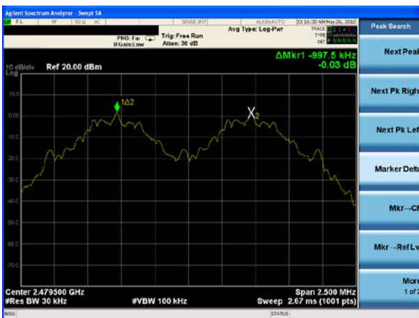
(1Mbps) Channel Separation plot on channel 77-78
