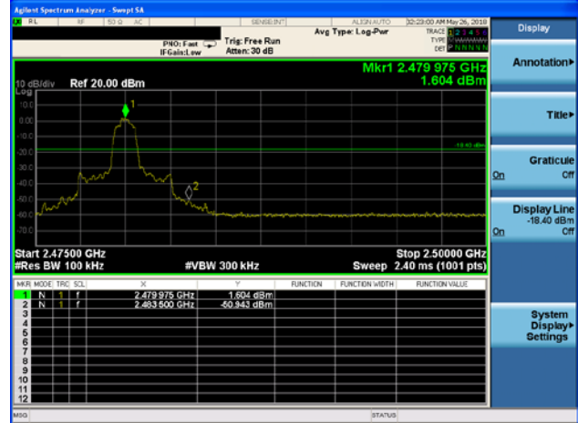
\pi/4 -DQPSK: Band Edge-High Channel (Hopping Mode)
