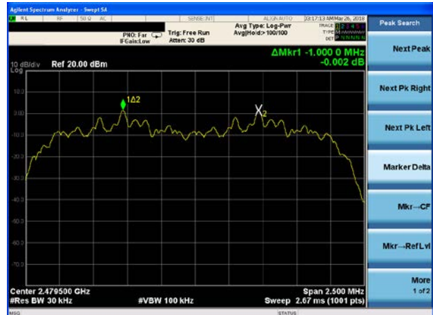
(2Mbps) Channel Separation plot on channel 77-78
