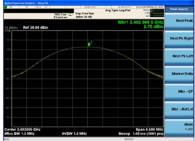
Peak output Power plot on channel 39 (2Mbps)
