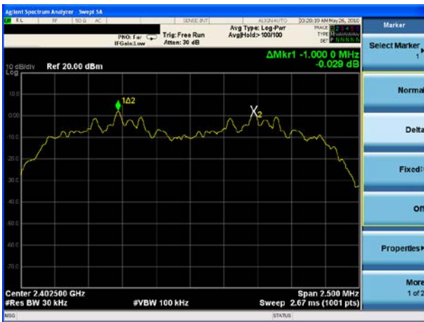
(3Mbps) Channel Separation plot on channel 39-40
