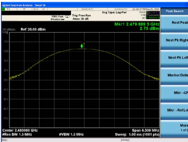
Peak output Power plot on channel 78 (3Mbps)
