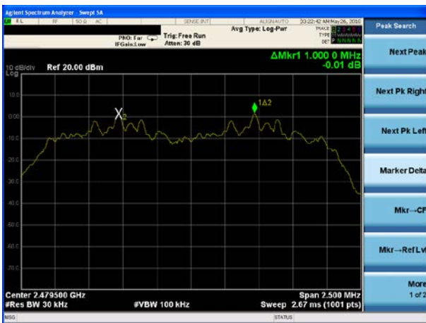
(3Mbps) Channel Separation plot on channel 77-78
