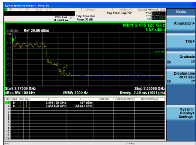
8-DPSK: Band Edge-High Channel (Hopping Mode)
