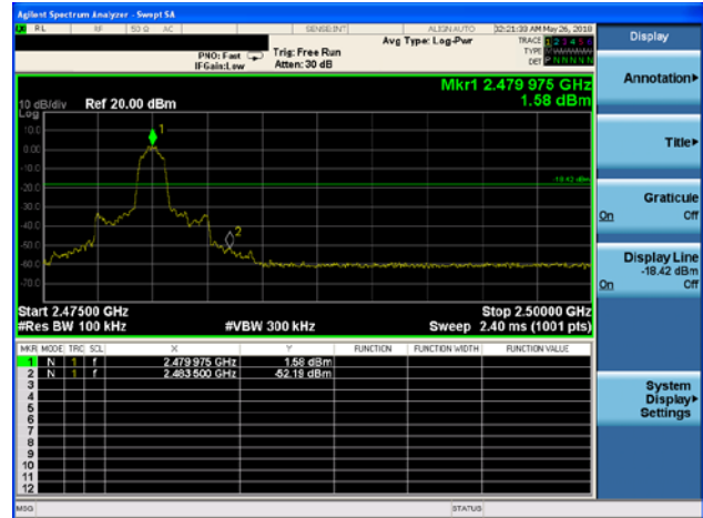
8-DPSK: Band Edge-High Channel
