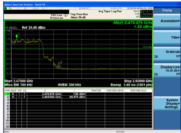
\pi/4 -DQPSK: Band Edge-High Channel (Hopping Mode)
