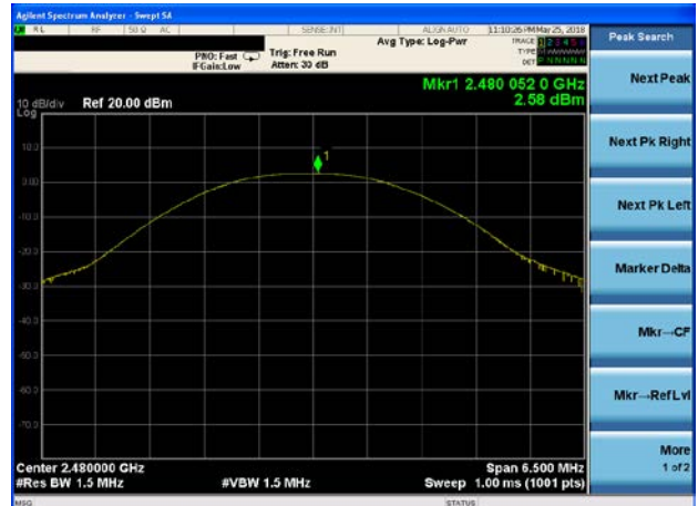
Peak output Power plot on channel 78 (2Mbps)
