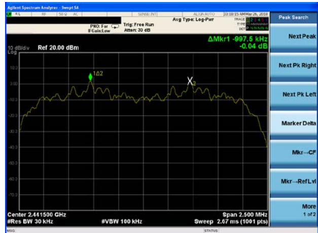
(2Mbps) Channel Separation plot on channel 39-40
