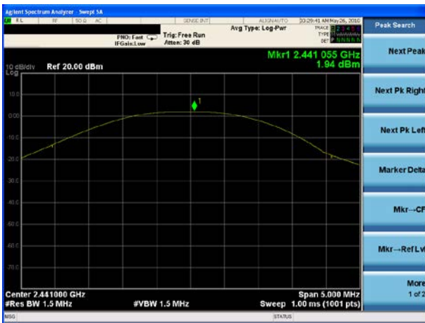
Peak output Power plot on channel 78 (1Mbps)
