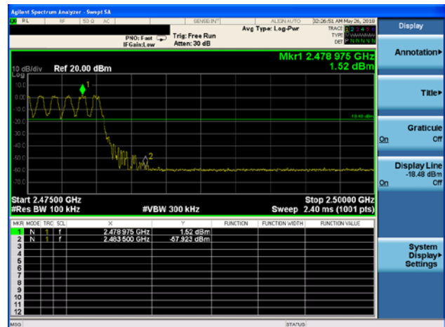
GFSK: Band Edge-High Channel (Hopping Mode)
