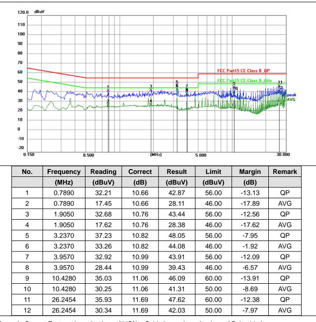
Remark: Correct Factor = Insertion loss of LISN + Cable loss + Insertion loss of Pulse Limiter; Measurement Result = Reading Level +Correct Factor;
