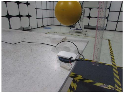
Note: The dummy load must be placed horizontal of the EUT at the top.(Parallel to the coil) ====END====
