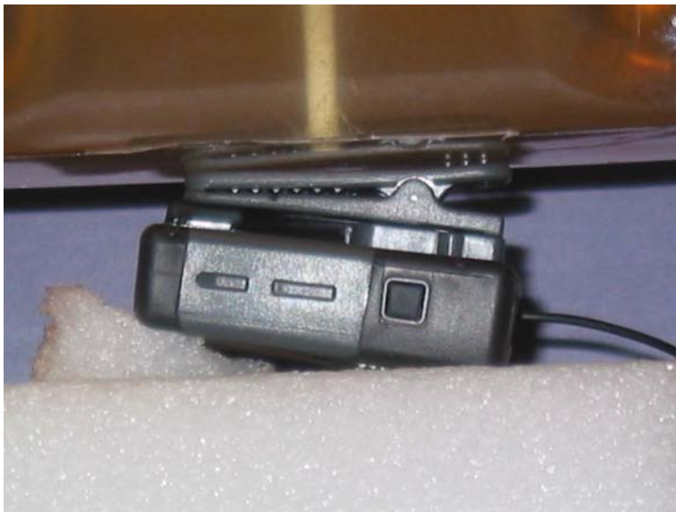
Test Position With Small Belt Clip and Lapel Mic 0 mm Gap
