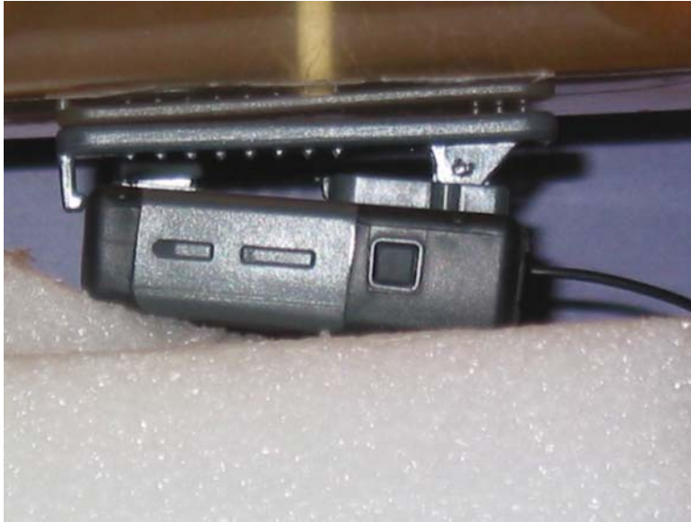
Test Position With Large Belt Clip and Lapel Mic 0 mm Gap
