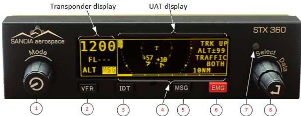
Figure 21: STX 360 front panel functionality
