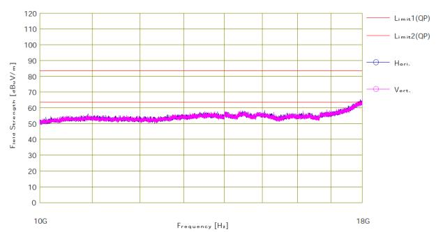
$\begin{array}{lll} Note \ 1: & Measured \ distance: 1 \ m \\ Note \ 2: & Limit: Peak: 83.5 \ dB \mu V/m \\ & Average: 63.5 \ dB \mu V/m \end{array}$
