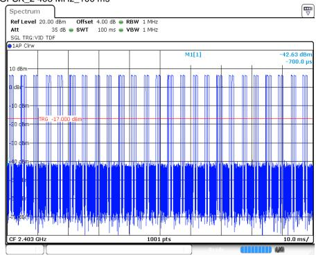
Worst case actually duty cycle : (4.050  $^{\ast}$  6) + (0.486  $^{\ast}$  2) / 100 = 0.253 Dutycycle Factor : 20log(0.253) = -11.9 dB Note 1:
