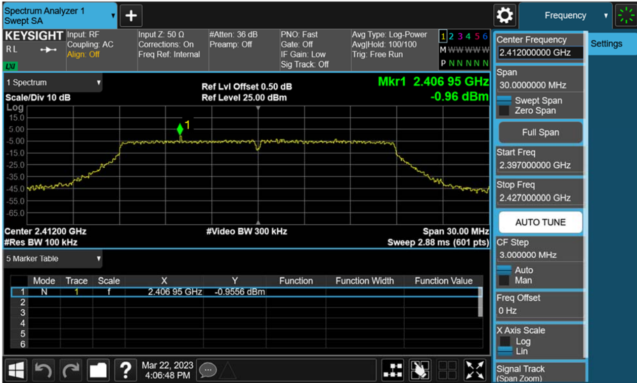
Figure 31: Conducted Spurious Emission & Authorized-band band-edge, 802.11n(HT20), 2412MHz Carrier Level
