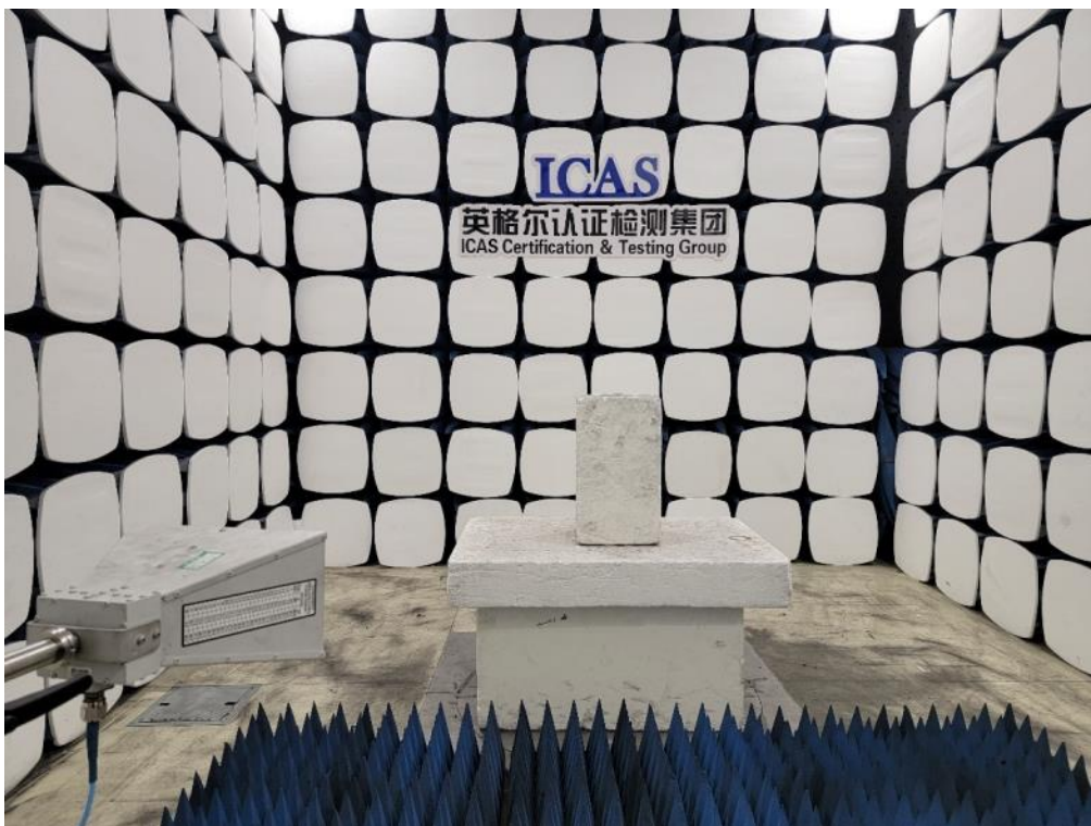
FCC Radiated Emission Test Setup-above 1GHz
