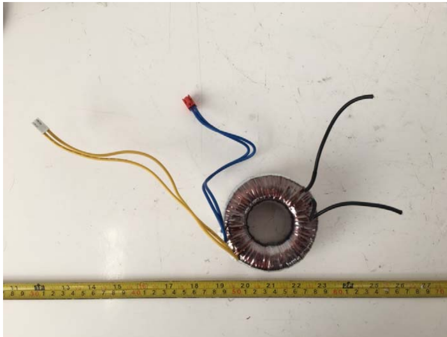
EUT –Transformer View-1
