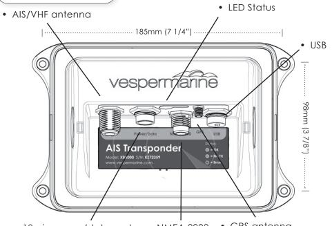
• 10 pin power/data port • NMEA 2000 • GPS antenna
