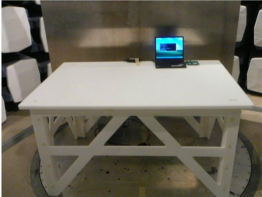
**19.6 AC Line Conducted Emission Side View**
