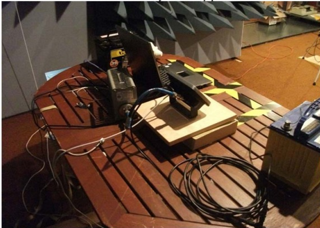
Radiated immunity test set up photos
