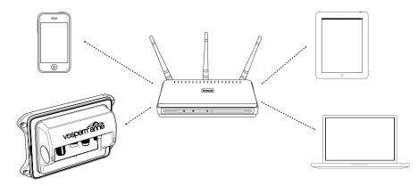
The XB-8000 can also join an existing network. It can do this in either DHCP mode (default) or you can set a static IP address using vmAIS (see configuration section). To prevent the address from automatically changinig we recommend that you use a static IP address.
