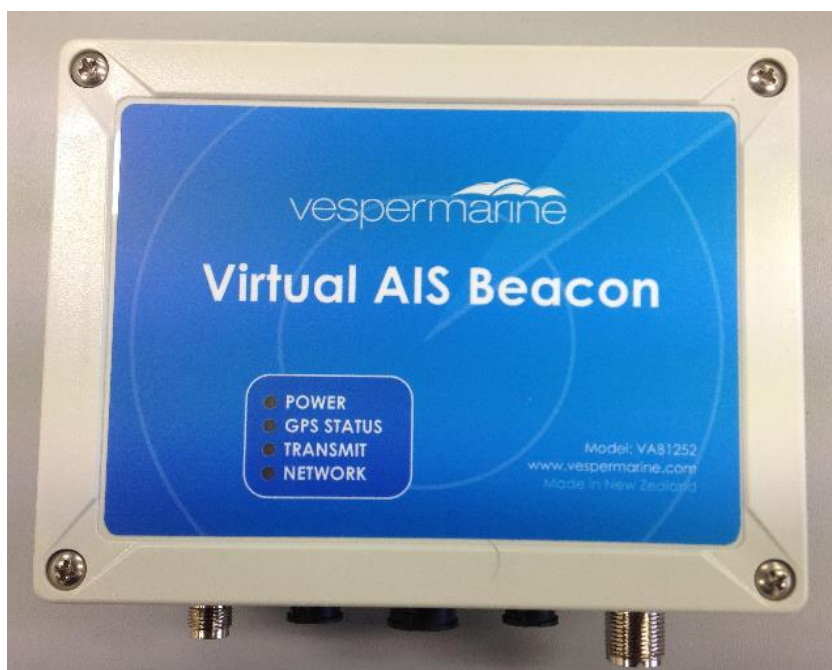
Virtual AIS Beacon Housing, Top - showing LED bank and main label
