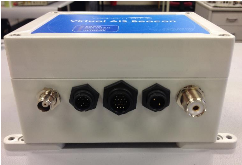
Virtual AIS Beacon Housing, Front - showing GPS, 10-pin, 16-pin, Power Supply and VHF connectors
