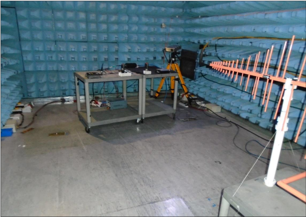
Figure 17 - Test Setup - Below 1 GHz
