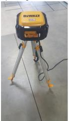
Press the feet of the tripod into the ground iv.
