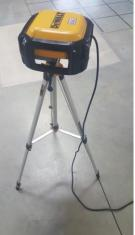
b. DW0737 Construction Tripod Mounting
