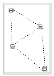
5. In a large open area stagger Access Point placement for best coverage and redundnacy. Install Access Point with the DEWALT Logo facing the floor when hung from the ceiling
